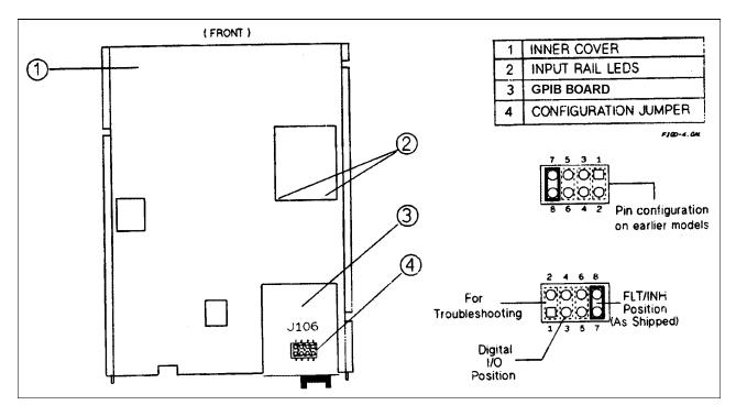
Figure D-4. Digital Port Configuration Jumper
